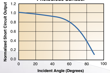
Normalized Output Current vs. Incident Angle of Light to Photodiode Surface.
